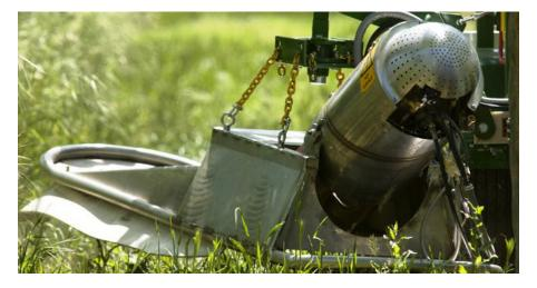
The new Batchen Stinger steam weed control machine is now being refined for the U.S. market. The Stinger generates and transfers an 800 degrees Fahrenheit steam to kill weeds.
